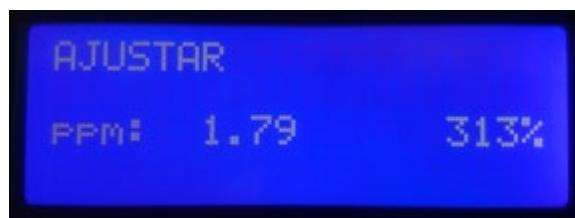
Return to the main screen. The current CL value will match with the value obtained from DPD-1 test.
