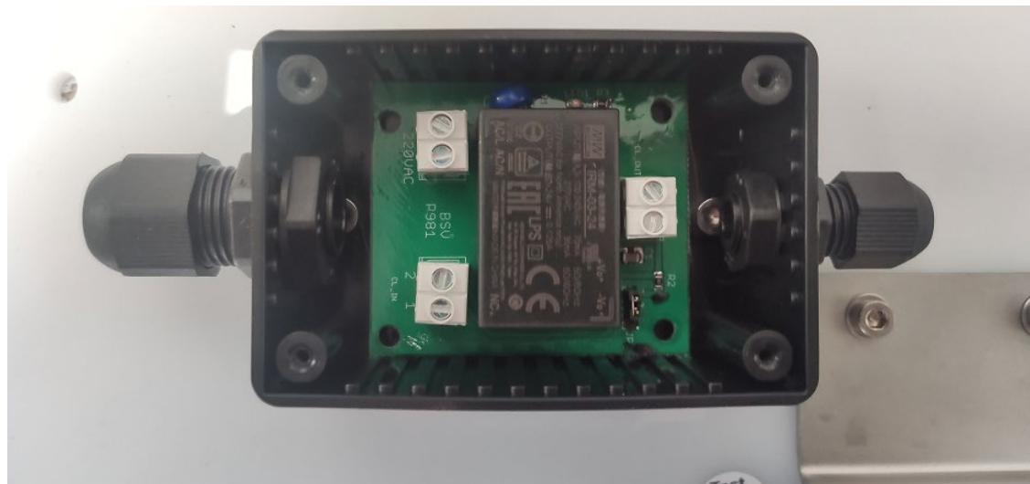
Connect the probe following the next diagram. This connection box must be also connected to the 220V AC mains.
