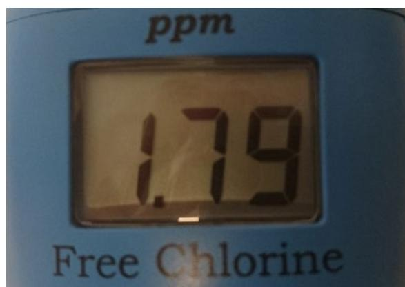
Chlorine Menu -> Select “calibration” and press OK. Wait until the reading is stable:
