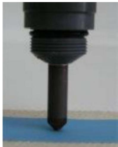
Carefully wash the header with tap water and fill it again with new electrolyte. In case of the header needs to be replaced, discard the used and install a new one.
