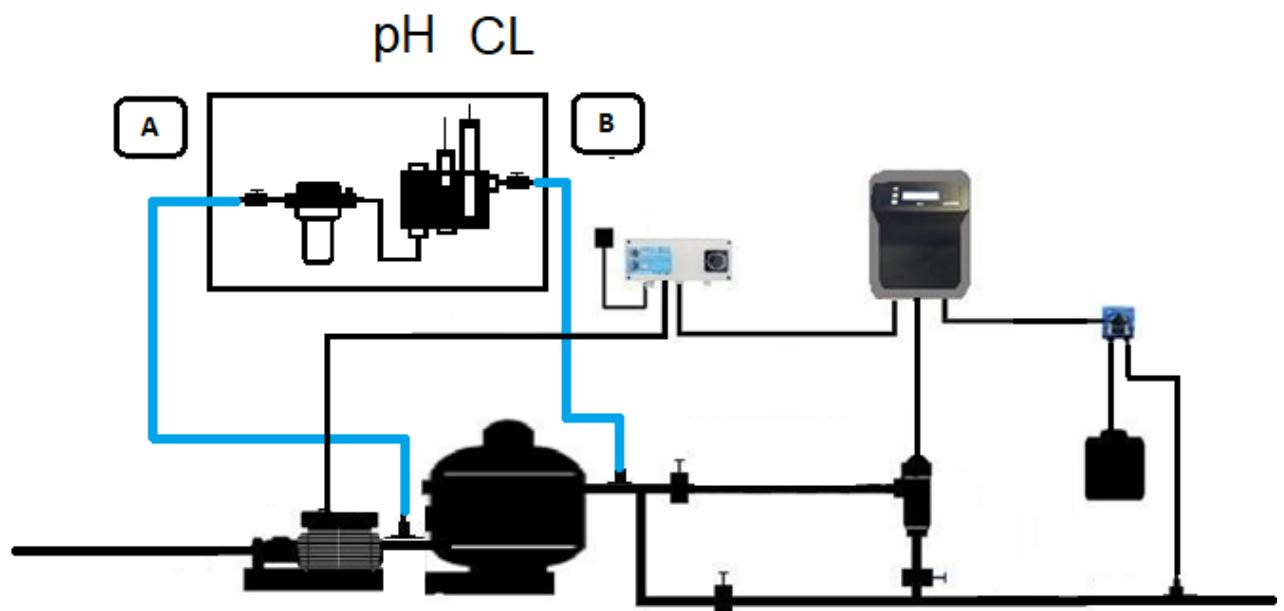
Install the panel on the wall, and connect the water inlet "A" to a pipe water sampling point, after the filtration pump.
