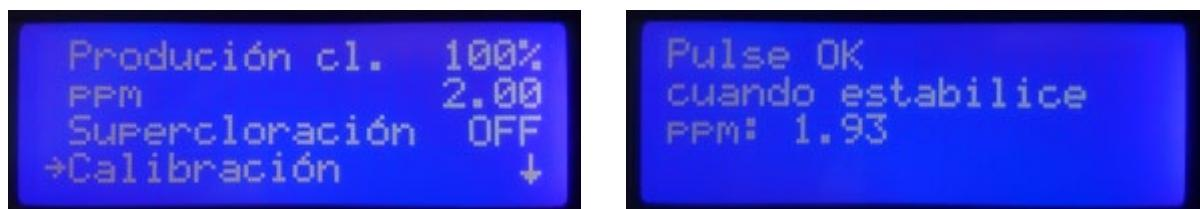
Adjust the real value obtained by means of DPD-1 test.
