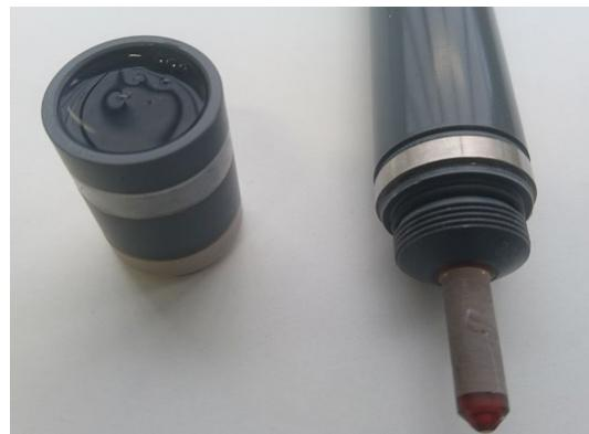
**Caution:** Before screwing again the header cap to the sensor body, the silicone ring must be removed, uncovering the small hole shown in the following picture:
