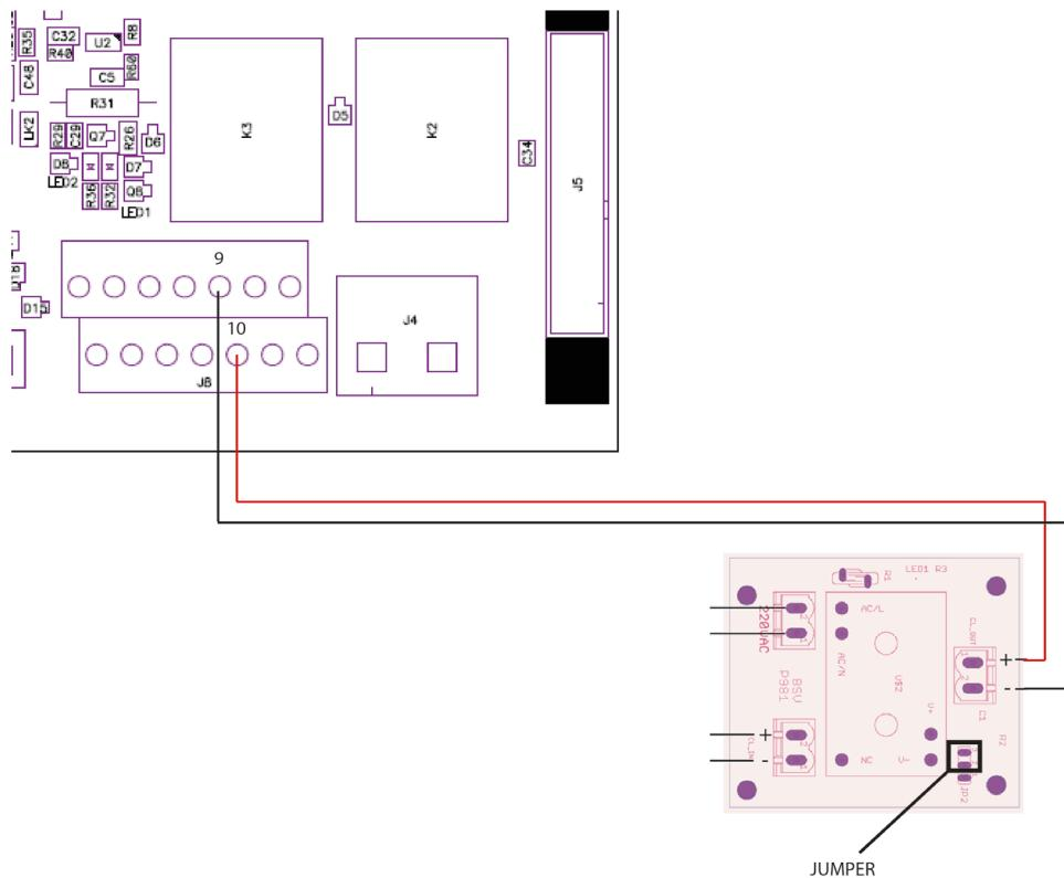
Connection with PRO200-1000 salt water chlorinator series:
